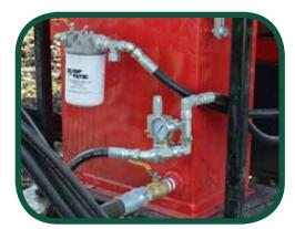
If speed is what you need, an onboard PTO-driven hydraulic system can cut your unload time by up to 33%.
