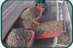
35-ton ( $32 \text{ MT}/48 \text{ m}^3$ ) capacity will quickly and efficiently build a clamp or fill a truck.
